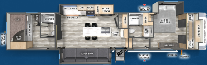
35CRIB LENGTH 42' 8" WIDTH 96" HEIGHT 13' 6" UVV 11,953 LB GVWR 14,305 LB HITCH 2,305 LB CCC 2,352 LB AWNING 10' 6" & 14' FRESH 60 GAL GRAY 76 GAL BLACK 76 GAL
