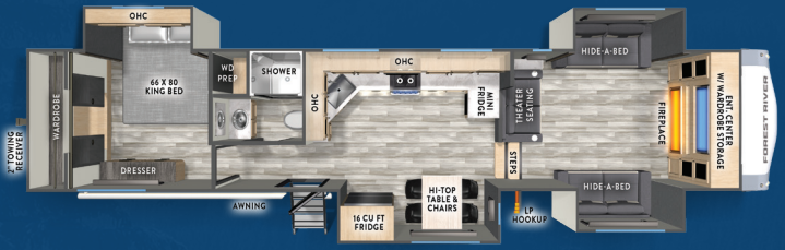
35FL LENGTH 43' 5" WIDTH 96" HEIGHT 13' 2" UVV 10,708 LB GVWR 14,115 LB HITCH 2,115 LB CCC 3,407 LB AWNING 15' FRESH 60 GAL GRAY 76 GAL BLACK 38 GAL
