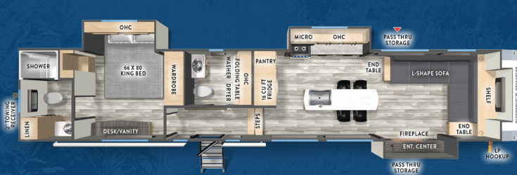
37PUB LENGTH 42' 9" WIDTH 96" HEIGHT 13' 5" UVV 10,873 LB GVWR 14,050 LB HITCH 2,050 LB CCC 3,177 LB AWNING 19' FRESH 60 GAL GRAY 76 GAL BLACK 76 GAL
