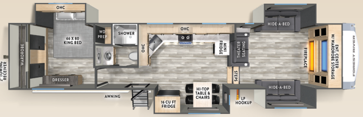
35FL LENGTH 43' 5" WIDTH 96" HEIGHT 13' 2" UVW 10,708 LB GVWR 14,115 LB HITCH 2,115 LB CCC 3,407 LB AWNING 15' FRESH 60 GAL GRAY 76 GAL BLACK 38 GAL
