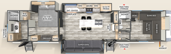
36FUN LENGTH 42' 9" WIDTH 96" HEIGHT 13' 5" UVW 12,033 LB GVWR 14,095 LB HITCH 2,095 LB CCC 2,062 LB AWNING 13' & 12' FRESH 60 GAL GRAY 76 GAL BLACK 76 GAL
